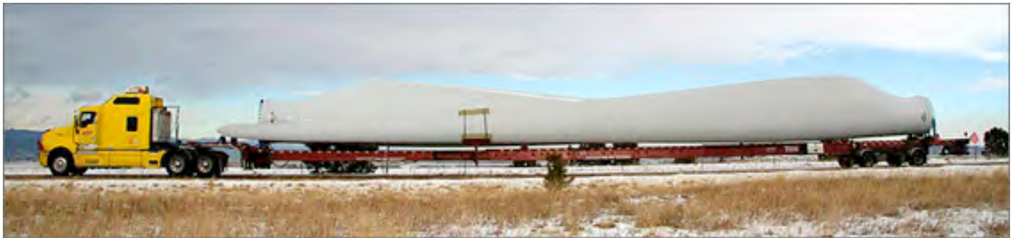
Fig. 7. Photo of a long truck parked on a road with a yellow cab and red trailer carrying a white wind turbine blade. Trucks capable of transporting wind turbine blades are some of the largest and heaviest vehicles driving on the nation's roadways. Delivery routes must be carefully planned and approved to avoid urban rush hours, narrow lanes, sharp curves and weak bridges. Credit: Jim Green
