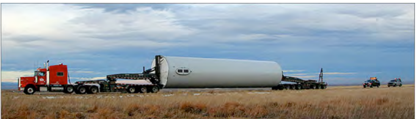
Fig. 9. A truck carrying a section of steel tower for a GE 1.5 MW wind turbine approaches the National Wind Technology Center. The truck has 13 axles to distribute the weight of its cargo. The escort vehicles behind have radio-controlled equipment to help steer the trailer from behind. Credit: Jim Johnson
