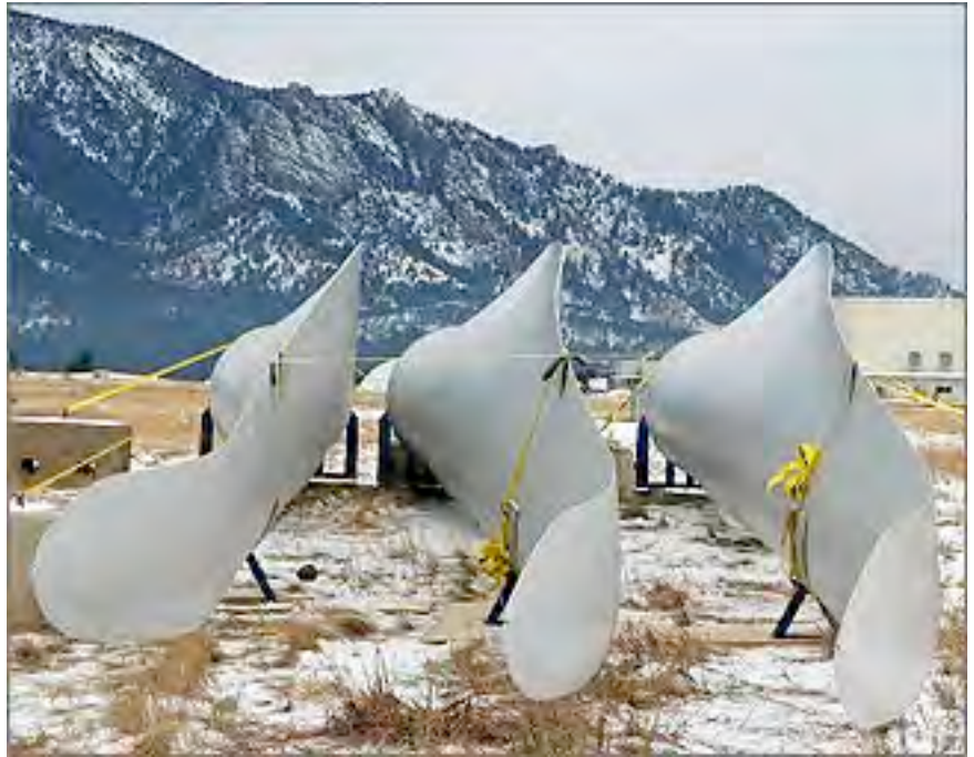
Fig. 6. Blades of the General Electric 1.5 MW turbine are being stored outside on cradles this winter at the National Wind Technology Center. They are secured with large concrete blocks to prevent them from being damaged during high winds and storms. Credit: Jim Green
