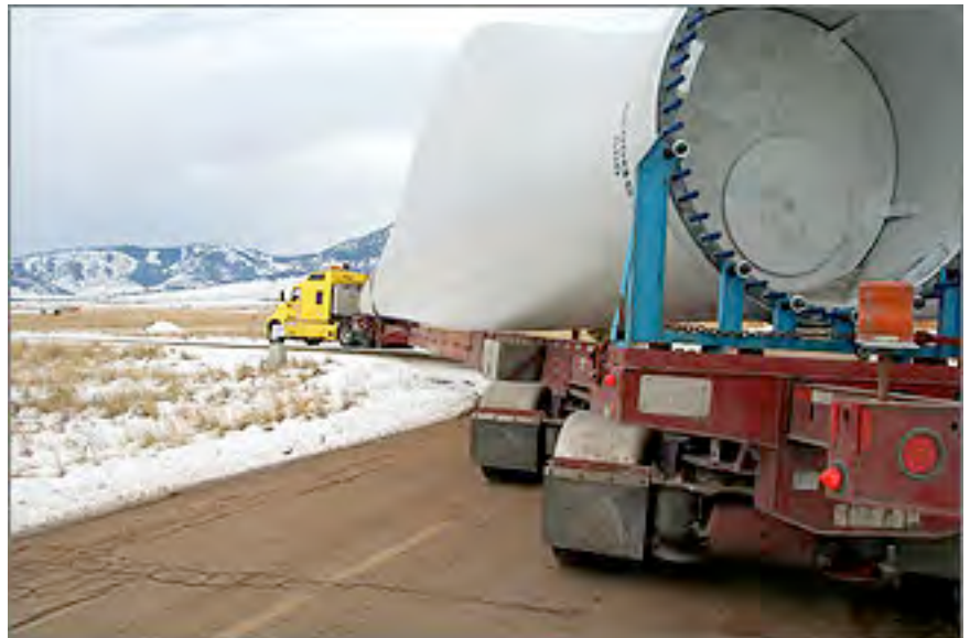
Fig. 8. A truck carrying a wind blade negotiates a sharp curve at the National Wind Technology Center. The logistics of delivering and installing increasingly large wind turbine components is just one issue that requires attention if the U.S. is to meet 20 percent of its electricity needs with wind power by 2030. Credit: Jim Green.
